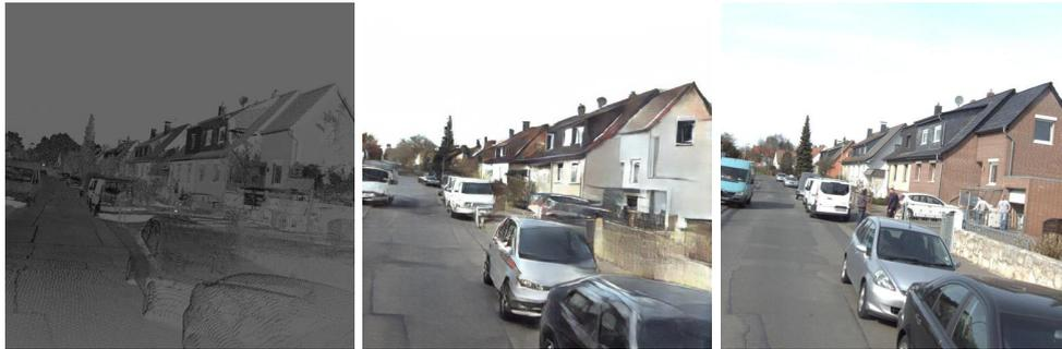
■ **Figure 3** Input image (reflectance, left), synthesized image (middle) and real image (right).
